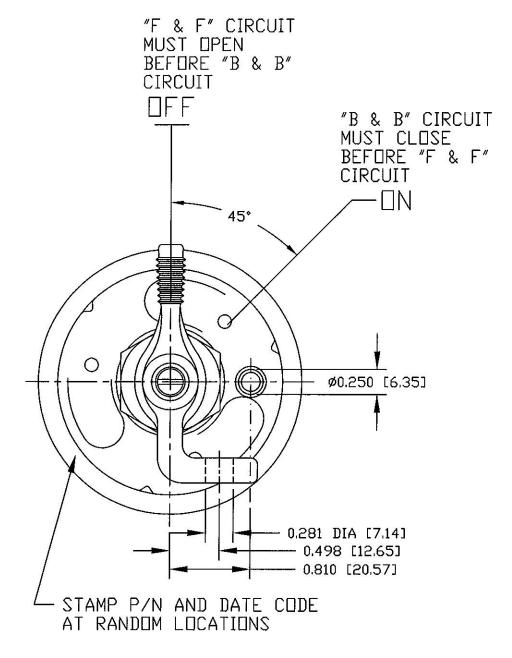
SCREW, #8-32 & LOCKWASHER, NOTE 4 - SHAFT — HEX NUT, 3/4-16, N□TE 4 LOCKWASHER, 2 REQ'D, NOTE 4 HEX NUT, 2 REQ'D, NOTE 4 LOCKWASHER, NOTE 4 -LOCKWASHER, 2 REQ'D, NOTE 4 0.335 [8.51] ---0.925 [23.50] UL LABEL 0.550 [13.97] -3.470 [88.13]
