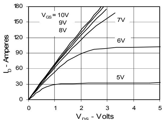
**Fig. 3. Output Characteristics
