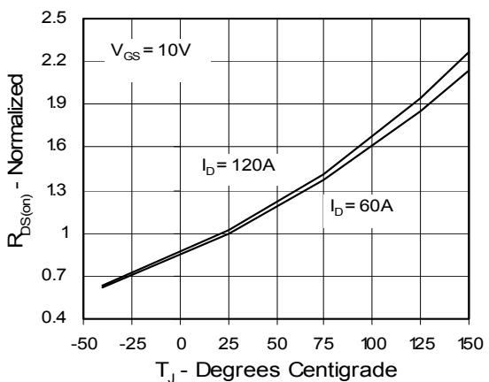
**Fig. 5.  $R_{DS(on)}$  Normalized to  $I_{D25}$
