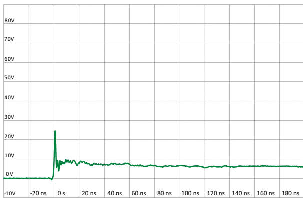
IEC 61000-4-2 +8 kV Contact ESD Clamping Voltage
