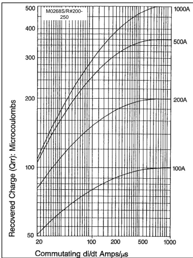
Figure 5 – Maximum recovered charge,  $Q_{ra}$  (50% chord)
