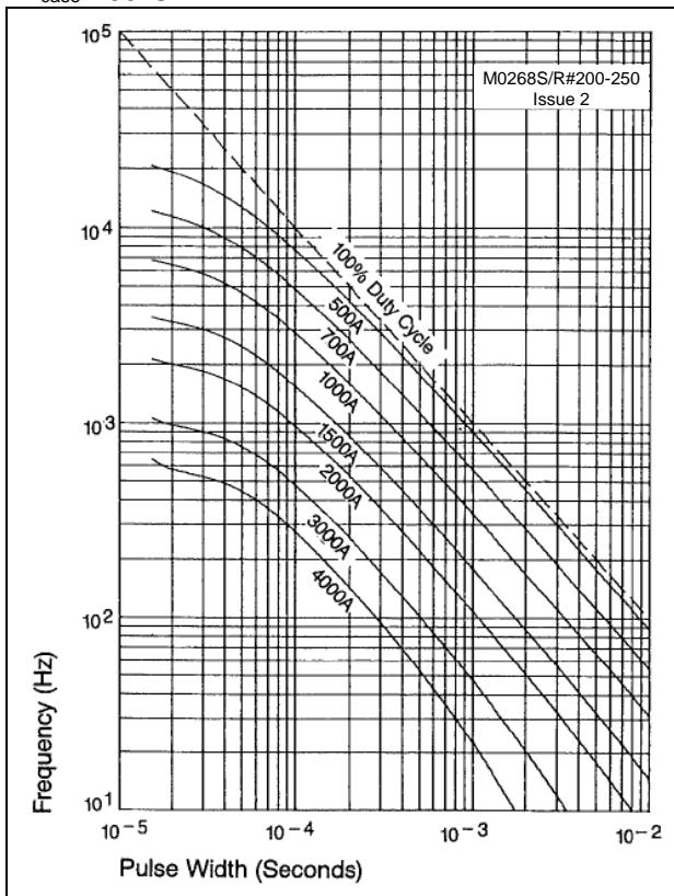
Figure 9 - Sine wave frequency vs. pulse width,  $T_{case}$  - 90°C
