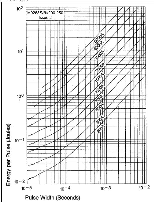
Figure 11 - Square wave energy per pulse, 800A/ $\mu$ s
