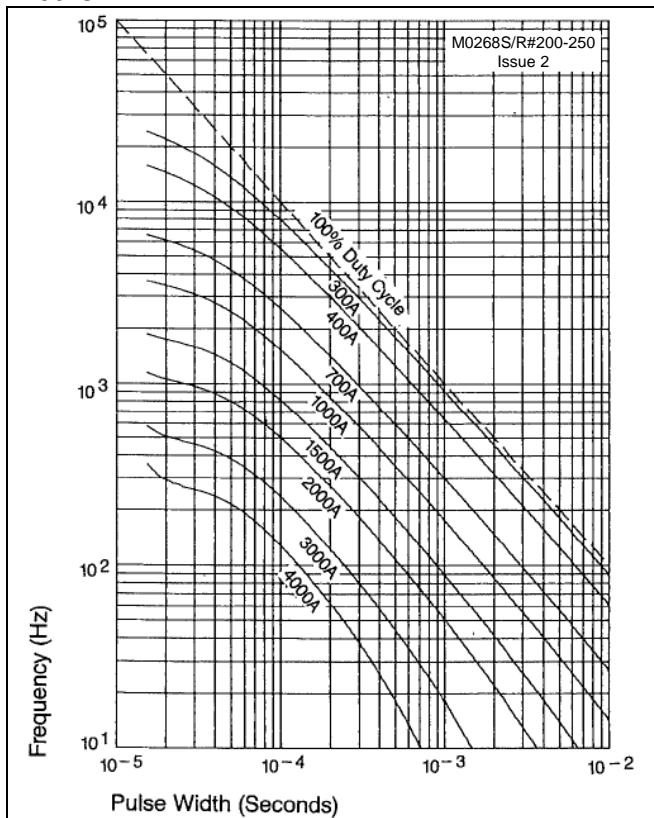
Figure 10 - Square wave energy per pulse,
