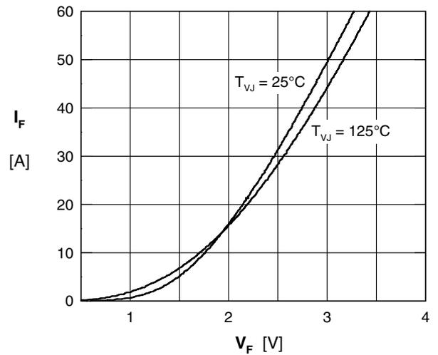
Fig. 19 Typ. forward characteristics of brake diode
