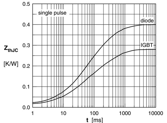
Fig. 16 Transient thermal impedance junction to case
