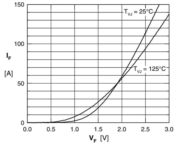
Fig. 10 Typical forward characteristic of free wheeling diode
