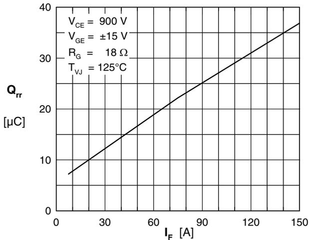
Fig. 15 Typical turn-off characteristics of free wheeling diode
