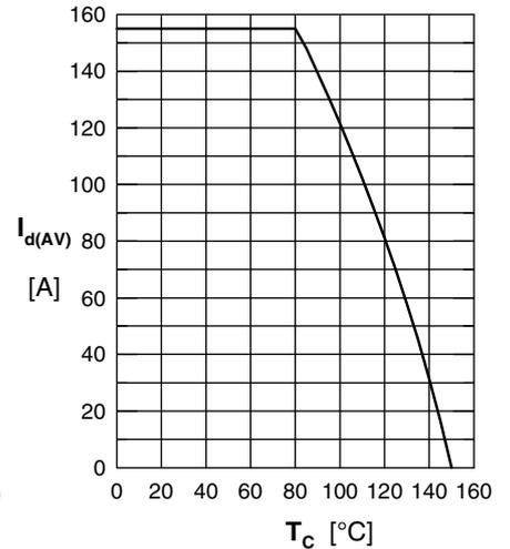
Fig. 5 Max. forward current vs. case temperature
