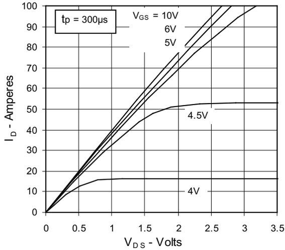
Fig. 1 Typ. output characteristics  $I_D = f(V_{DS})$
