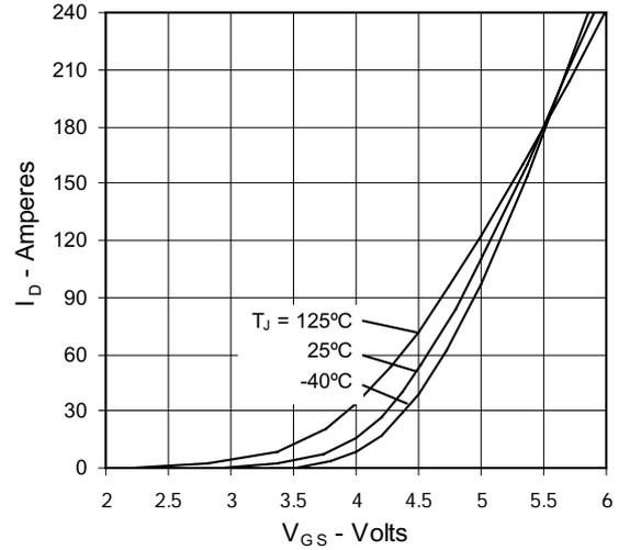
Fig. 2 Typ. transfer characteristics  $I_D = f(V_{GS})$
