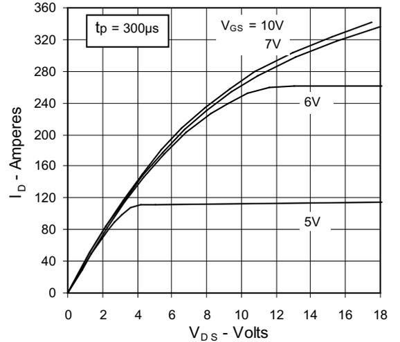
Fig. 8 Forward Safe Operating Area,  $I_D = f(V_{DS})$
