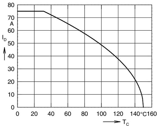
Fig. 5 Continuous drain current  $I_D = f(T_C)$
