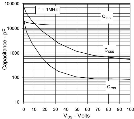
Fig. 9 Typ. capacitances  $C = f(V_{DS})$ ,  $f = 1 \text{ MHz}$
