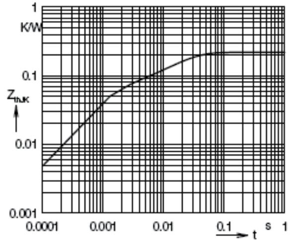
Fig. 12 Transient thermal resistance  $Z_{thJK} = f(t_p)$
