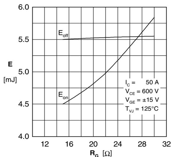
Fig. 6 Typ. switching energy vs. gate resistance
