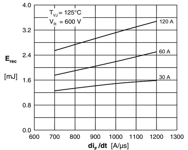
Fig. 8 Typ. recovery energy  $E_{rec}$  versus  $di/dt$
