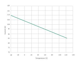
Rerating depicted in these curves is in addition to the standard derating of 25 % for continuous operating.
