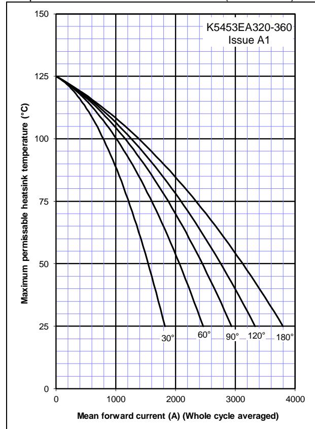
Figure 15 – On-state current vs. Power dissipation –
