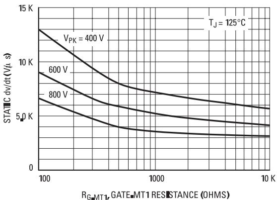
**Figure 11. Exponential Static dv/dt vs. Peak Voltage, MT2(+)**
