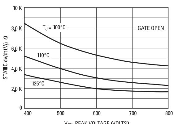
**Figure 12. Exponential Static dv/dt vs. Peak Voltage, MT2(-)**
