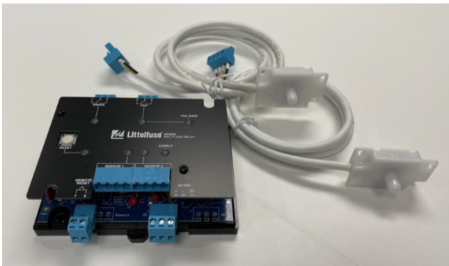
FIGURE 3. Littelfuse AF0025 arc-flash relay with two PGA-LS10-01B point sensors.
