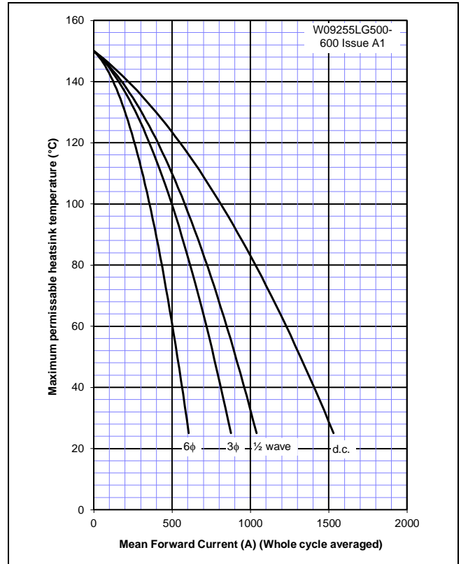
Figure 11 – Forward current vs. Heatsink temperature – Anode Side Cooled
