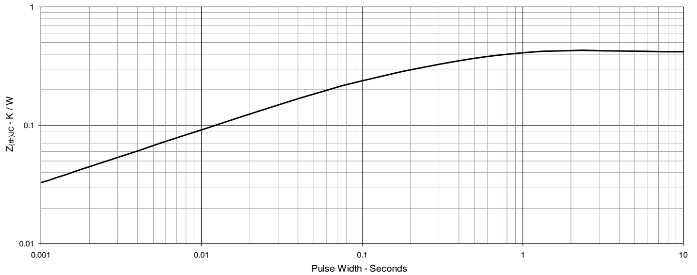
Fig. 13. Maximum Transient Thermal Impedance
