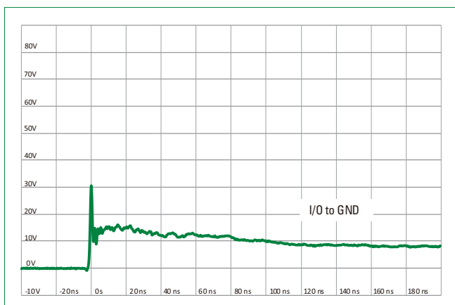
IEC 61000-4-2 +8 kV Contact ESD Clamping Voltage
