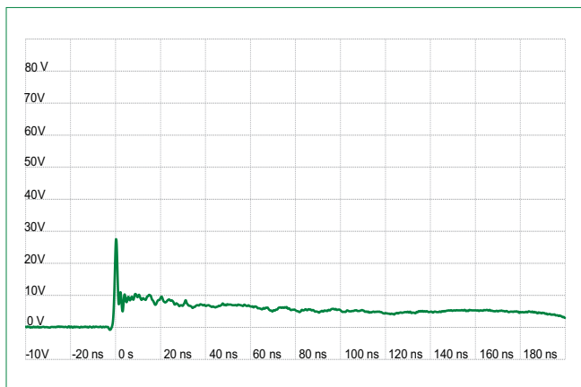
IEC 61000-4-2 +8 kV Contact ESD Clamping Voltage
