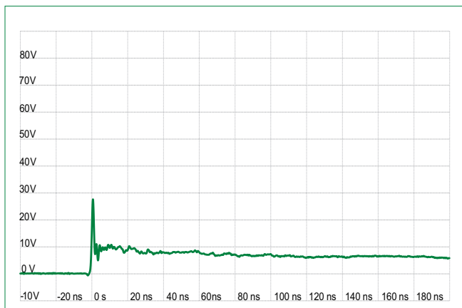
ISO10605 Contact Discharge Plot at +8 kV
