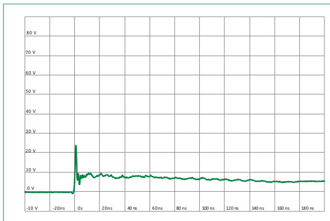
ISO10605 Contact Discharge Plot at +8 kV
