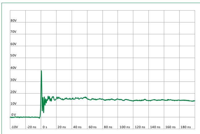
ISO10605 Contact Discharge Plot at +8 kV
