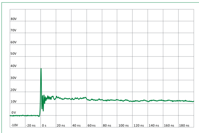
IEC 61000-4-2 +8 kV Contact ESD Clamping Voltage
