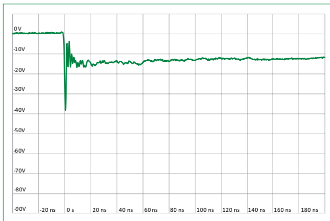
IEC 61000-4-2 -8 kV Contact ESD Clamping Voltage
