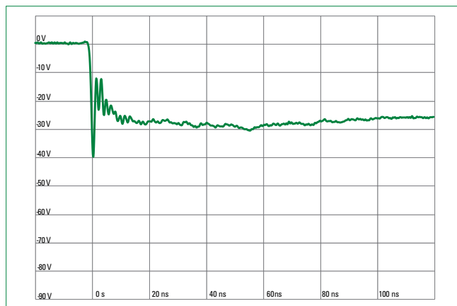
IEC 61000-4-2 -8 kV Contact ESD Clamping Voltage
