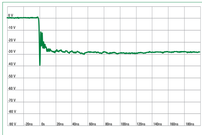
ISO10605 Contact Discharge Plot at -8 kV
