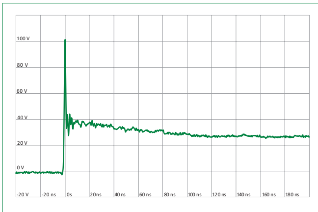
ISO10605 Contact Discharge Plot at +8 kV
