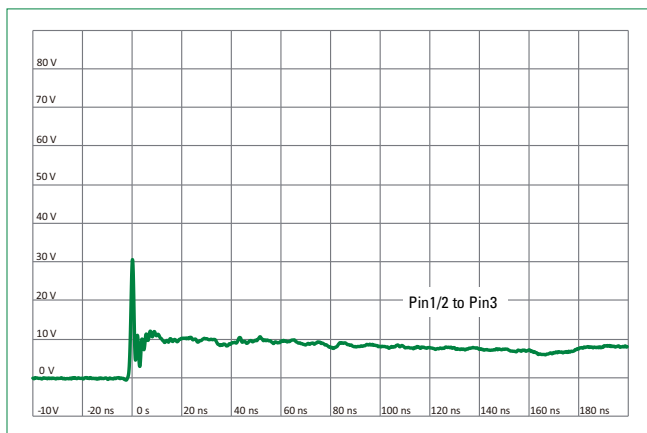
IEC 61000-4-2 +8 kV Contact ESD Clamping Voltage
