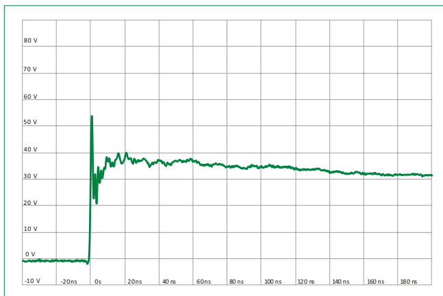
ISO10605 Contact Discharge Plot at +8 kV
