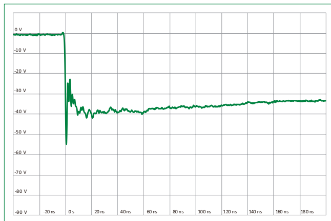
ISO10605 Contact Discharge Plot at -8 kV
