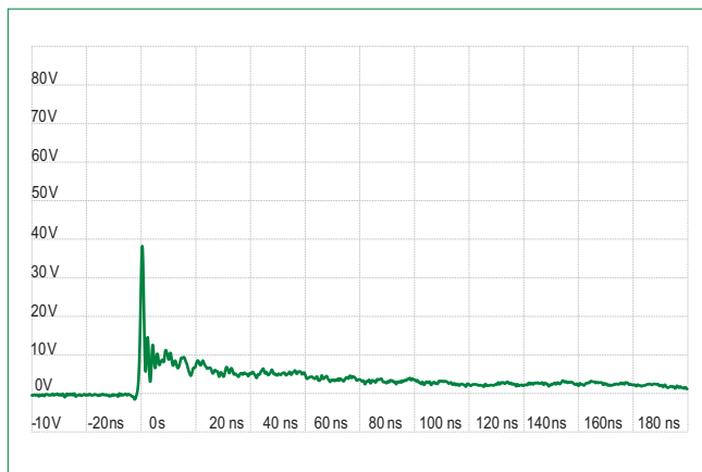
IEC 61000-4-2 +8 kV Contact ESD Clamping Voltage
