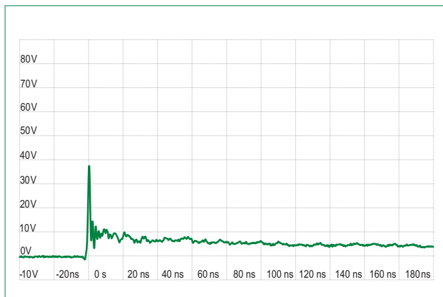
ISO10605 Contact Discharge Plot at +8 kV
