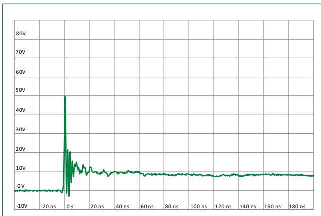
IEC 61000-4-2 +8 kV Contact ESD Clamping Voltage
