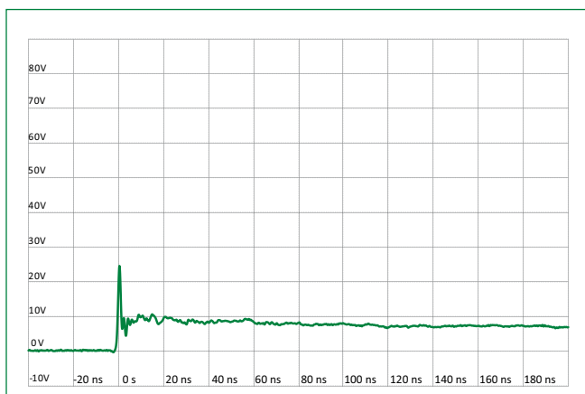
ISO10605 Contact Discharge Plot at +8 kV
