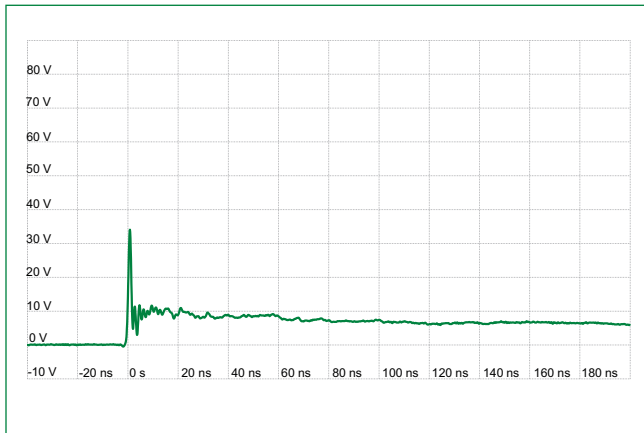
IEC 61000-4-2 +8 kV Contact ESD Clamping Voltage
