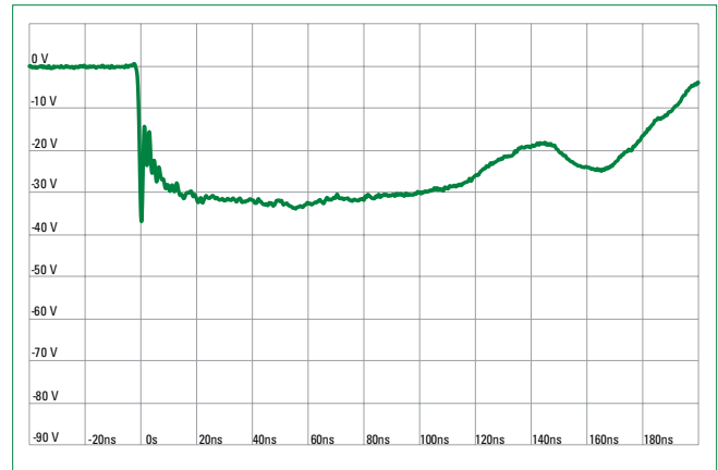
IEC 61000-4-2 -8 kV Contact ESD Clamping Voltage
