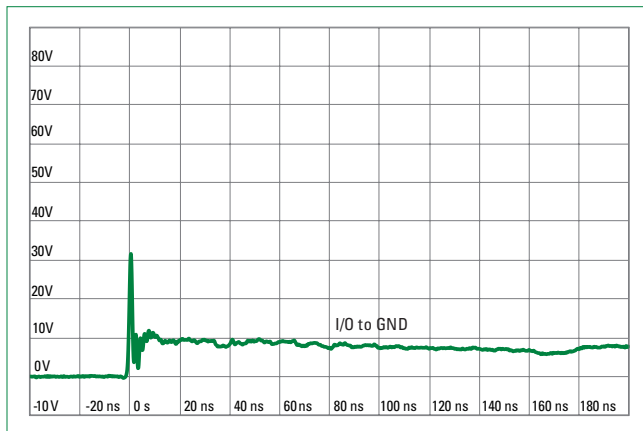
IEC 61000-4-2 +8 kV Contact ESD Clamping Voltage
