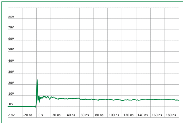
IEC 61000-4-2 +8 kV Contact ESD Clamping Voltage
