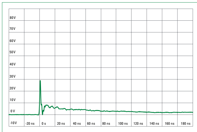
IEC 61000-4-2 +8 kV Contact ESD Clamping Voltage
