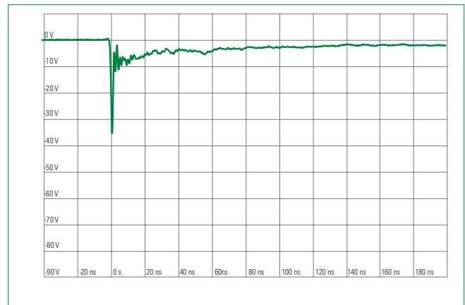
IEC 61000-4-2 -8 kV Contact ESD Clamping Voltage
