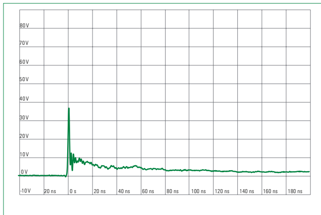
IEC 61000-4-2 +8 kV Contact ESD Clamping Voltage
