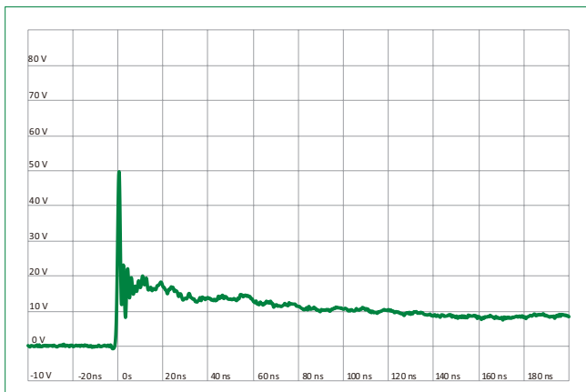
IEC 61000-4-2 +8 kV Contact ESD Clamping Voltage
