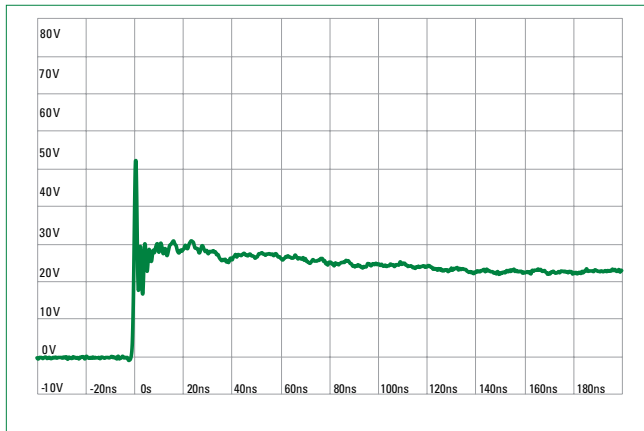
IEC 61000-4-2 +8 kV Contact ESD Clamping Voltage
