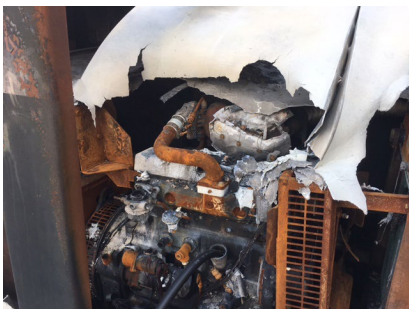
Mobile generator destroyed by arc-flash.
