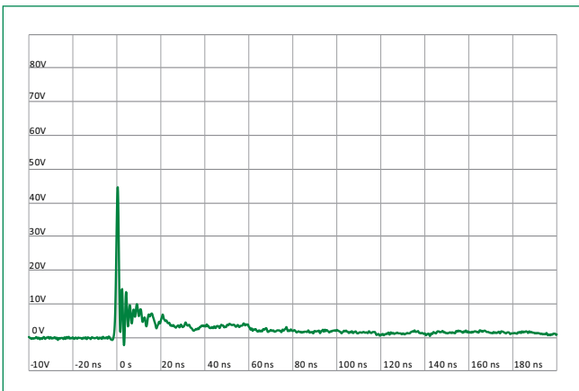
IEC 61000-4-2 +8 kV Contact ESD Clamping Voltage
