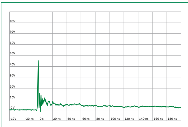
ISO10605 Contact Discharge Plot at +8KV
