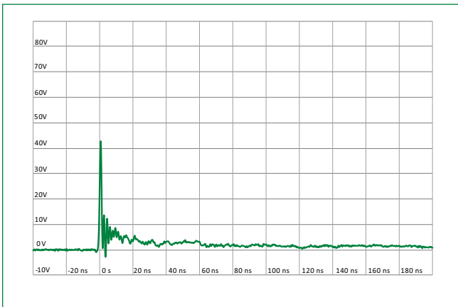
IEC 61000-4-2 +8 kV Contact ESD Clamping Voltage
