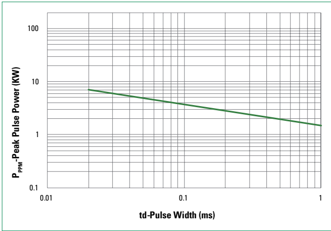
Figure 1 - Peak Pulse Power Rating Curve
