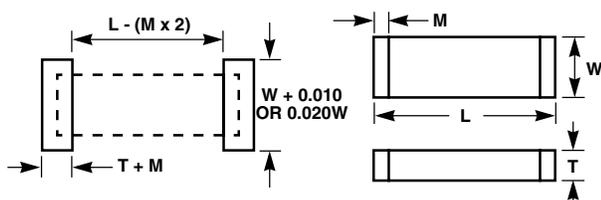
FIGURE 4. FORMULA FOR SURFACE MOUNTABLE VARISTOR FOOTPRINTS
