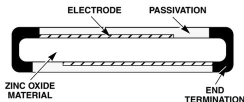
FIGURE 2. CROSS-SECTION OF THE "CH" SERIES OF METAL OXIDE VARISTORS
