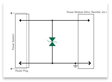
Using high-power TVS Diodes in a power supply configuration offer advantages over conventional methods, including no wear-out mechanism, faster response, and compact design.
