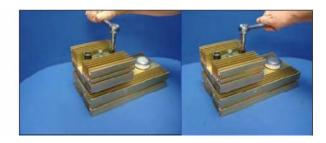
4. Check the top disc spring(s) after each bolt has been quarter turned. Correct force is applied when the washers are just free to move.
