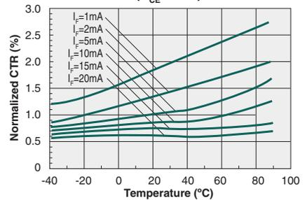
**Typical Transfer Characteristics of Darlington Transistor**
