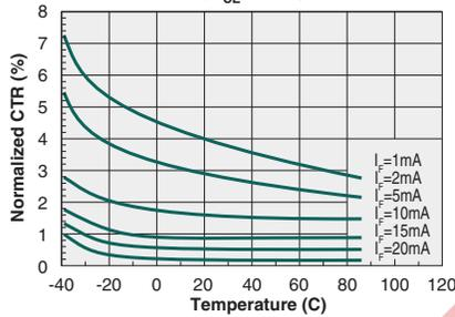
**Single Transistor Normalized CTR vs. Forward Current ( $V_{CE}=0.5V$ )**
