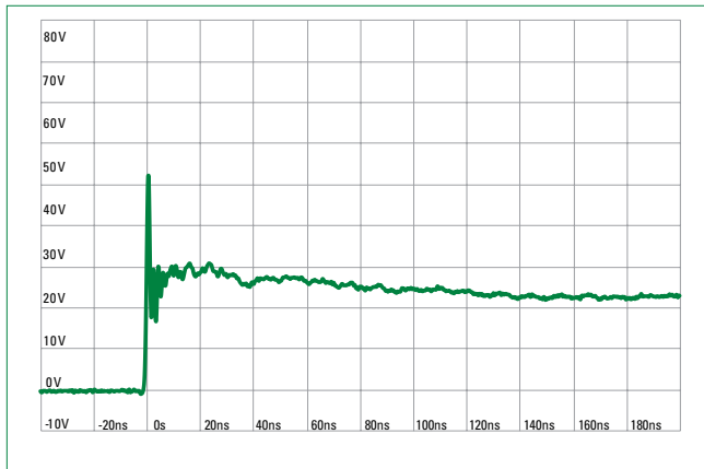
IEC 61000-4-2 +8 kV Contact ESD Clamping Voltage
