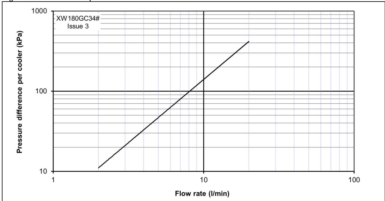
Figure 3 – Pressure drop vs Water flow
