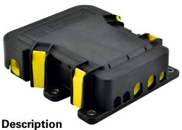
Sealed high current power distribution box using MIDI® and MEGA® type fuses. Designed to handle standard voltage (32V) and the new 70V (48V application) MIDI® and MEGA® fuses. Built for rugged environments, the MDB5 not only provides IP67/69K fuse sealing, but also seals all input and output connections.
