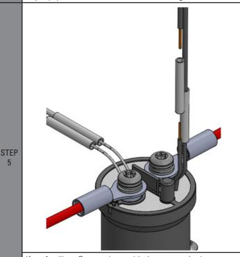
If an Auxiliary Contact is provided, connect the low power Line feed wire to one of the black wires and the low power Load output wire to the remaining black wire. When installing the wires, be sure that a good electrical connection is made. Do not allow any loose strands to short against any equipment and cause electrical damage.
