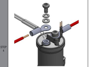
Verify the switched contacts are open, no continuity between terminals "A1" and "A2" Using the hardware that is supplied with the contactor or the recommended fasteners, connect the Line power feed wire to the contactor terminal marked "A1". Connect the Load power output wire to the contactor terminal marked "A2". As with the control wires, be sure that a good electrical connection is made. Do not allow any loose strands to short against any equipment and cause electrical damage.
