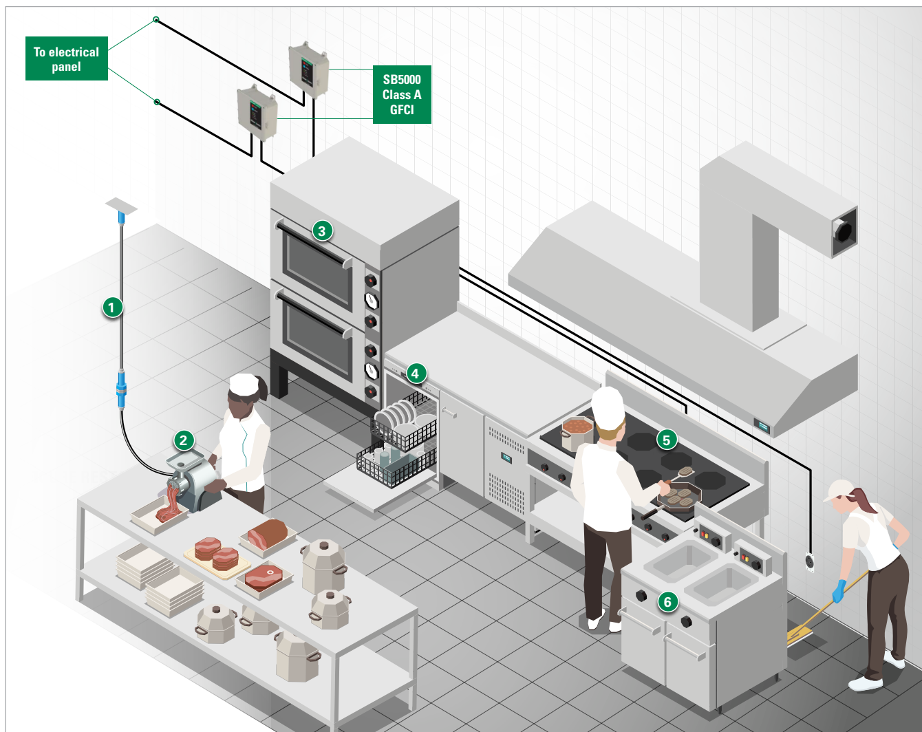
1 Drop-Down Receptacles for Prep 2 Meat Grinder 3 Electric Oven/Pizza Oven 4 Dishwasher 5 Electric Range 6 Deep Fryer
