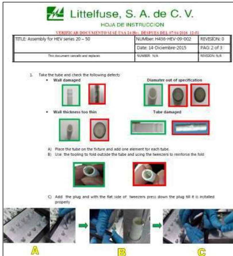
Figure 26 - Example of work instruction.
