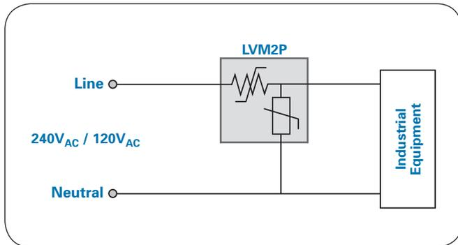
Figure 1 : Typical circuit diagram utilizing the 2Pro LVM2P-015R10431 device
