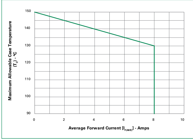
Figure 3: Maximum Allowable Case Temperature vs. Average On-State Current
