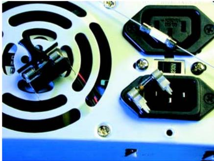
currents up to 150A at 250V. Miniature fuses are typically mounted into holders so they can easily be replaced. Shocksafe holders are available in PC Mount and Panel Mount versions. Open types such as clips or blocks offer a lower cost alternative. Additionally, you can directly
