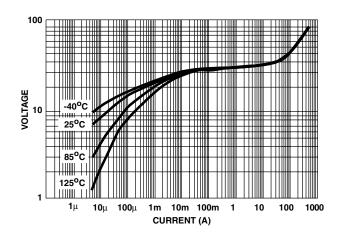
FIGURE 9. TYPICAL V - I CHARACTERISTICS OF THE V18AUMLA2220 AT -40°C, 25°C, 85°C AND 125°C
