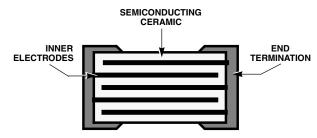
FIGURE 4. AUML INNER CONSTRUCTION
