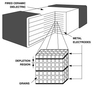
FIGURE 3. AUML TRANSIENT VOLTAGE SUPPRESSOR
