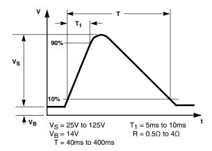
FIGURE 2. LOAD DUMP TRANSIENT
